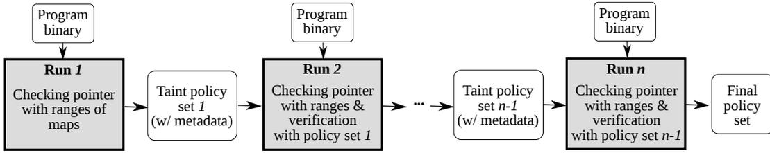
**Fig. 3:** The work-flow of multi-run pointer verification. For each policy, the metadata indicates which registers/memory is written to. Only pointers that point to the same relative address throughout multiple runs are kept.
