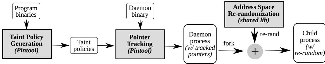
**Fig. 2:** An overview of RUNTIMEASLR’s architecture. It consists of three components: taint policy generation, pointer tracking, and address space re-randomization. Program binaries include the daemon binary.
