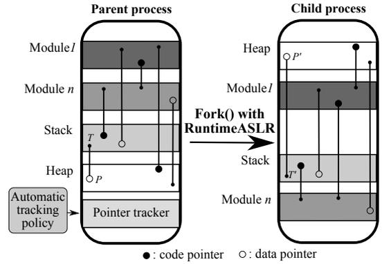
**Fig. 1:** **RUNTIMEASLR** approach for re-randomization with `fork()`. Pointer tracker accurately tracks all pointers based on automatically generated tracking policy set. Module-level re-randomization is performed and all pointers are updated for `fork()`. For example, in parent process, a pointer  $P$  in heap points to  $T$  in stack. After the re-randomization, stack is moved and thus  $T$  is moved to  $T'$ . Accordingly,  $P$  is patched to  $P'$ .
